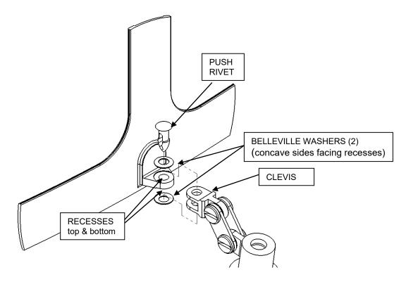
Position Belleville washers in recess of mounting ear. Engage clevis of headlight into place. Align parts and push plastic rivet into place.
